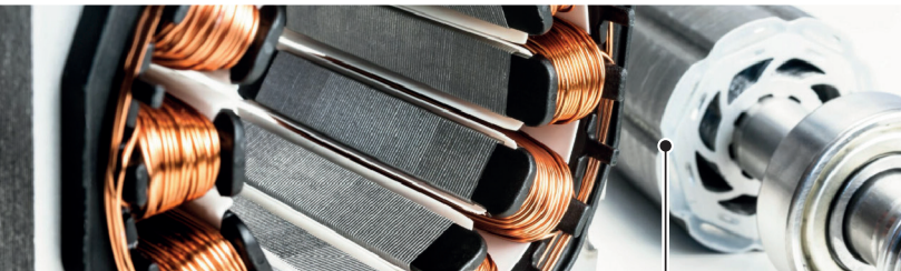
EV motor: Magnetic rotor spins in changing electrical field
