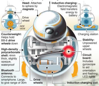
Two electric motors: These power two *drive wheels* independently, allowing them to turn in different directions and make BB-8 rotate
