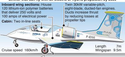
Undercarriage: Two retractable wheels and two small wheels under wings. 6kW electric motor accelerates aircraft up to 60km/h during take-off
