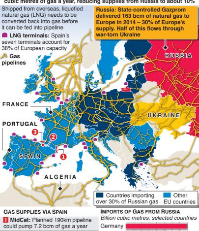
2 Larrau: Main connection with France upgraded last year, increasing capacity of pipeline to 5.2 bcm
