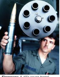
Firepower: A-10's seven-barrel 30mm GAU-8 Avenger rotary cannon can fire up to 70 rounds per second and disable enemy tanks at range of over 6,500m
