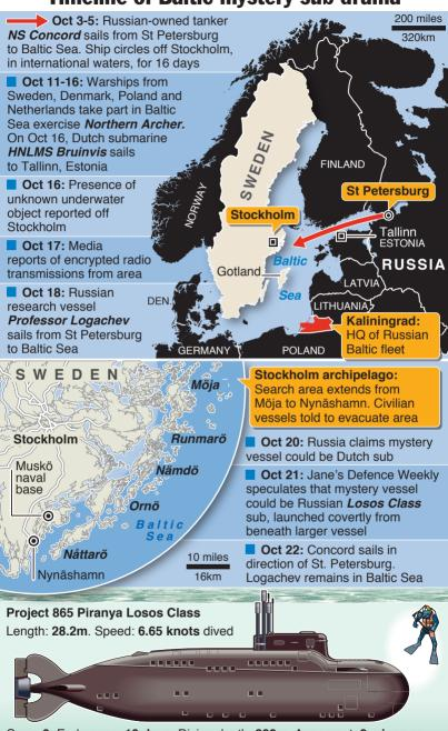
Crew: 9. Endurance: 10 days. Diving depth: 200m. Armament: 2 mines or 2 torpedoes. Titanium alloy hull reduces effectiveness of enemy mines
