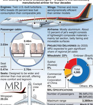
Typical cruising speed Mach 0.78 Fuselage (828km/h) length 33.4m (MRJ70) Pratt & Whitney PW1200G, Engines 35.8m (MRJ90) up to 78.2kN thrust Unit cost \$42 million Introduction Summer 2017 Height
