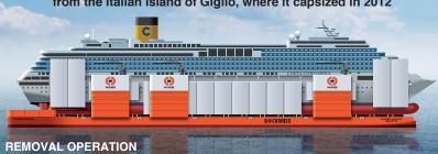
Wreck of Costa Concordia re-floated using air-filled caissons (metal boxes) attached to sides
