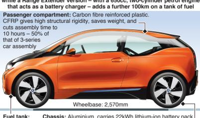
Fuel tank: Chassis: Aluminium, carries 22kWh lithium-ion battery pack and 125kW (170hp) electric motor to drive rear wheels
