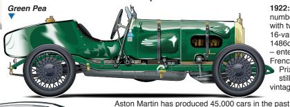
**1922:** Chassis number TT1 with twin cam, 16-valve, 1486cc engine entered in French Grand Prix. Car is still raced in vintage events
