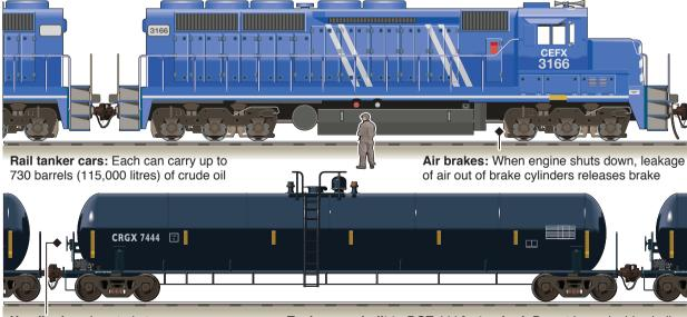
Handbrakes: Located at rear of each car. Large wheel is turned manually to lock wheels of car Tanker cars built to DOT-111A standard: Do not have double shells or shields of cars used for propane, and so are more likely to rupture and leak in event of derailment
