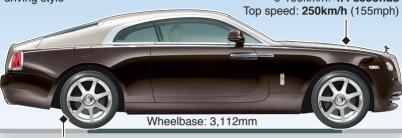
Suspension: Double-wishbone front and multi-link rear. Load calculations made by dampers every 2.5 milliseconds
