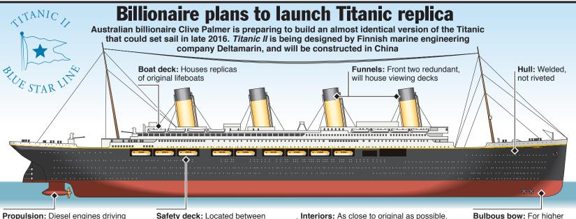
azimuth thrusters will replace original coal-fired steam engines
