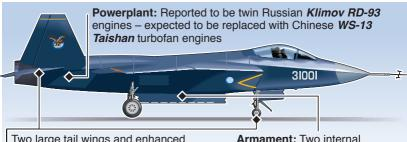
Two large tail wings and enhanced double-wheel nose landing gear suggest J-31 may be deployed from aircraft carrier
