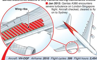
Feb 5: Plane grounded in Sydney after further precautionary inspection finds 36 hairline cracks on wing rib brackets. They are similar to "Type 1" cracks found in previous A380 checks
