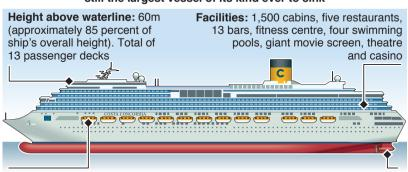
**Lifeboats:** Fully enclosed, engines operate even if boat is inverted
