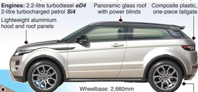
Ability to ford 500mm of water, 25 degree MagneRide: Magnetically approach angle, 210mm ground clearance
