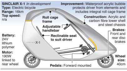
Length: 2.1m Width: 69cm Height: 1.4m Weight: 30kg
