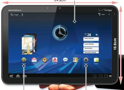
■ Connectivity: Wi-Fi, 3G, Bluetooth. Upgradeable to 4G. Micro-USB and mini-HDMI ports ■ Cameras: 2MP front-facing for video calling, 5MP rear-facing with dual LED flash. Also shoots HD video
