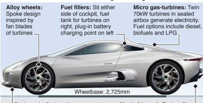
Bodywork: Carbon fibre wrapped around lightweight aluminium chassis. Up to 50% of metal is recycled
