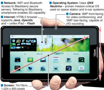
Connectivity: Micro-USB Processor: Dual-core 1GHz ARM
