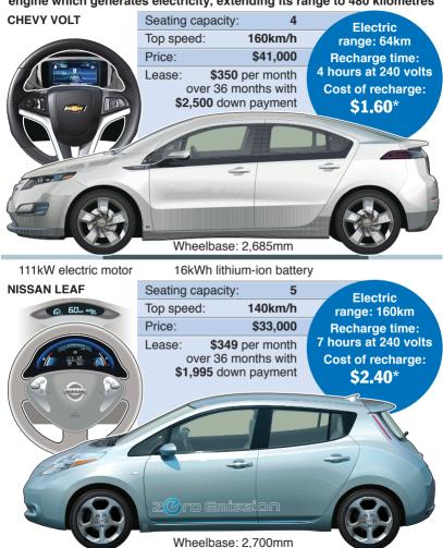
80kW electric motor 24kWh lithium-ion battery
