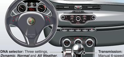
Dynamic, Normal and All Weather, modify operating parameters of engine, gearbox, steering system, O2 electronic differential and VDC
