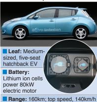
Charge time: 8 hours using 200V outlet or up to 80% charge in under 30 minutes using DC 50kW charger
