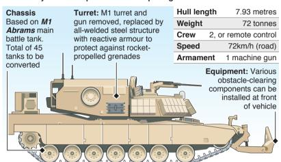
Breacher digs path through minefield using 4.5m-wide plough supported by skis that glide over ground If there are too many mines, rockets with explosive charges can be fired over 100m forward, detonating bombs at safe distance
