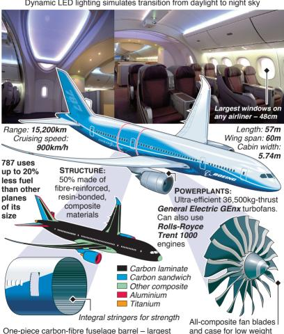
composite pressure vessel ever made – replaces 1,200 sheets of aluminium and 40,000 rivets
