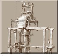
▲ 1801: French silk weaver Joseph Marie Jacquard patented a loom which used punch cards to control a sequence of operations, enabling the weaving of intricate patterns
