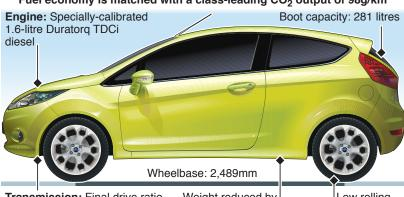
Transmission: Final drive ratio increased from 3.37 to 3.05.
