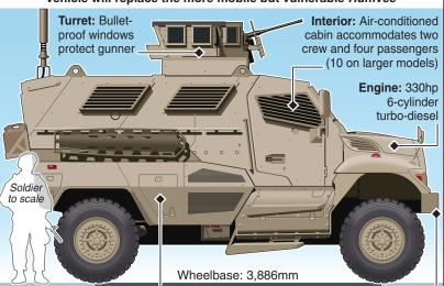
Armour: Thick armour plate integral to design unlike Humvee add-on kits
