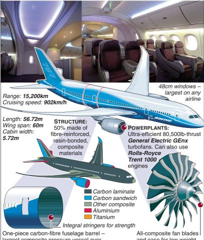
largest composite pressure vessel ever made – replaces 1,200 sheets of aluminium and 40,000 rivets
