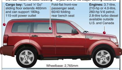
Drivetrains: Rear-wheel drive, part-time 4-wheel drive or full-time 4WD
