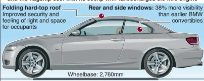
Mechanism: Three roof pieces fold away in 22 seconds at push of button in car
