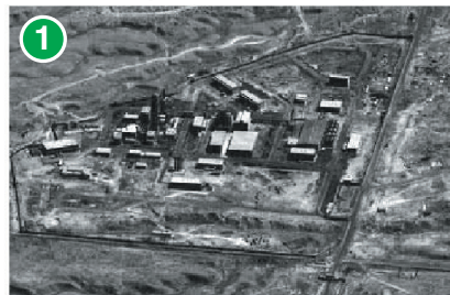
1. Project Baiji, al-Sharqat: Large new well-guarded chemical complex built at site of former uranium enrichment facility. Designed to produce nitric acid which can be used in the purification of uranium
